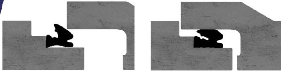
Apply lubricant to the whole surface around the pipe spigot before assembly. Pay special attention to the front edge of the spigot.
