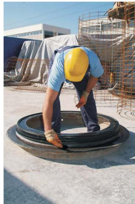
SECIL Integrated seal stretch on the cleaned and lightly oiled base ring. Ensure correct seating and even pre-stretching of the sealing ring. Before vibrating ensure that the socket is completely filled with concrete. Then produce concrete pipe in normal manner.
